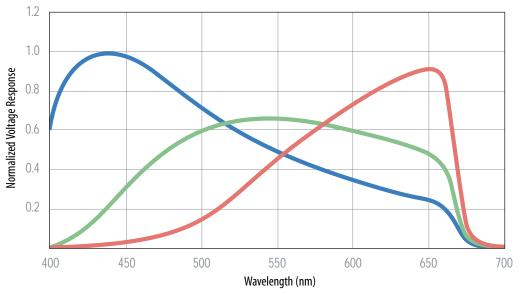
$^{\ast}$  IR filter (50% transmission at 660nm +/- 10nm) used for spectral sensitivity measurements.
