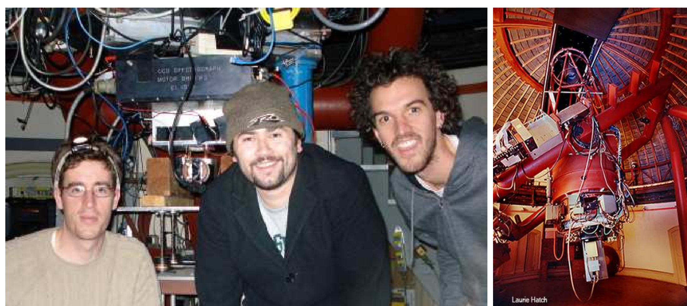
Figure 1: NB, JSB, and JS in front of our small camera (Left Figure), mounted to the Cassegrain focus of the Nickel 1 m telescope (Right Figure) at Lick Observatory.
