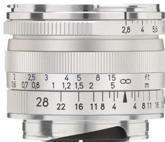
Figure 5. A Zeiss Ikon 28mm lens with depth-of-field scale. The hyperfocal distance appears to be about 1100mm at f/22 , on 35mm format, which implies a relative COC criterion of c = (28/43.3)(28/22)/1100 = 1/1350 . Other Zeiss lens images that I have examined, including medium format lenses, imply c values between 1/1533 and 1/1040, with one exception.
