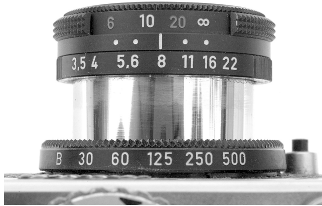
Figure 6. The actual Carl Zeiss Triotar 40mm f/3.5 lens from which David Jacobson measured C = 0.025 mm or c = 1/1730 (photo by David Jacobson). Interpreting the right-most dot as the f/16 far point at infinity, and the hyperfocal distance as about 13 feet or 4000 mm, we can confirm his numbers: C = (40/16)(40/4000) = 0.025 ; c = (40/43.3)(40/16)/4000 = 1/1730 . The most notable property of this lens is its low cost due to its simple three-element construction; why the COC is so tight is a bit of a mystery.
